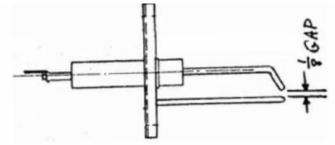
Reinstall assy and test water heater in propane mode by turning on the water heater switch inside. If furnace doesn't fire up and no popping sound is heard indicating that electrode is firing then either igniter is bad or water heater control module has failed
