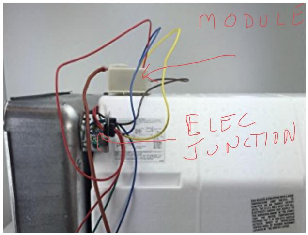
The control module is seen in this pic and is easy to replace. Take pics of where all the wires are attached. Remove defective module and order replacement module.. install module using pic you took BEFORE you removed wires and install wires.
