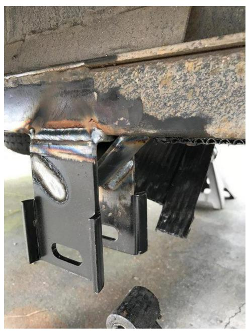
This bracket is for the Lippert Correct Track mounted spring eyes... The Dexter spring hanger doesn't have the lipped edges and the hole is not slotted like shown above
