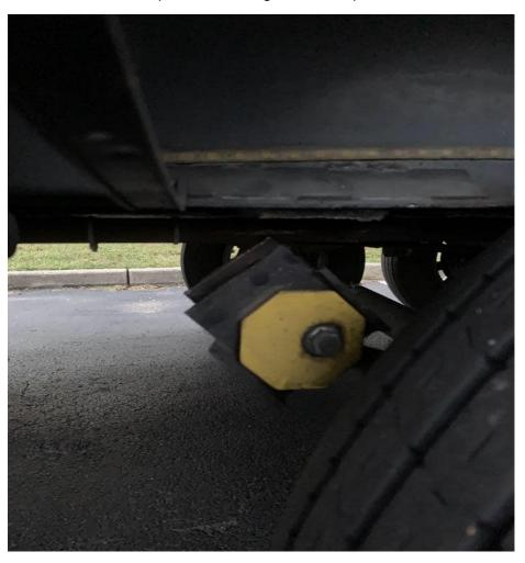
One more image of a broken spring hanger bracket .. this one is on a Non Lippert Correct track spring mount.. Typical Dexter assy like on my Alpine
