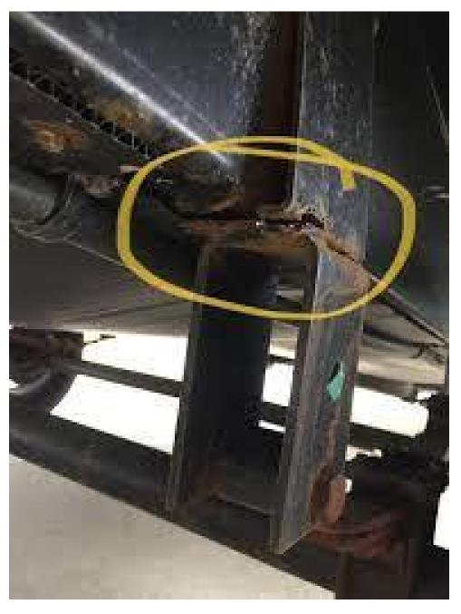
Here are a few images of Lipperts Spring hanger brace welded in place.. The images are from some Grand Design fifth wheels made in 2021 and later.. This is now a <u>Standard Option on some GD models</u>
